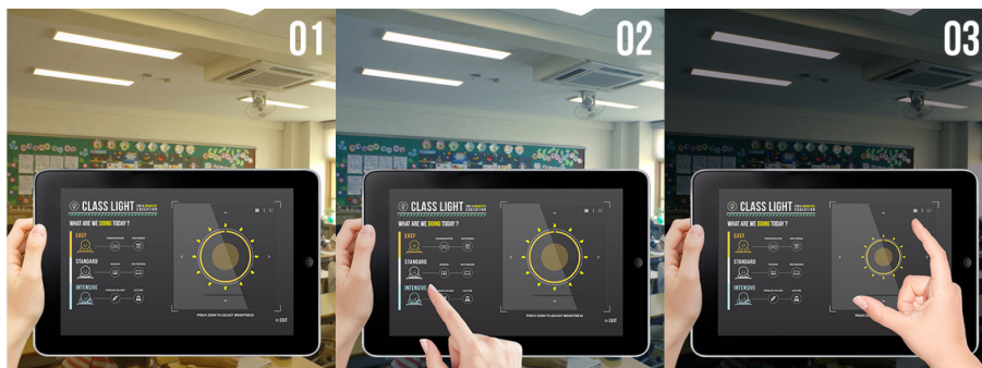
Fig. 6. Operational flow of the dynamic lighting system: 1) students are focusing on solving mathematical problems; 2) select the “intensive” lighting preset to support students’ academic performance; and 3) lower the illuminance level by pinching in the intensity icon for high intensity of daylight.
