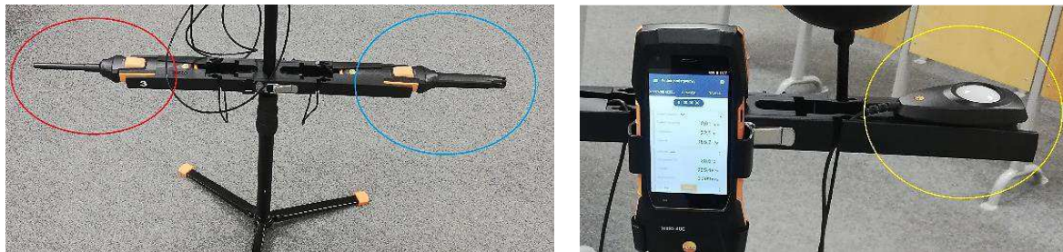
Fig. 2: Probes for collecting information on: CO 2 concentration (red circle), air temperature and humidity (blue circle) and light intensity (yellow circle).
